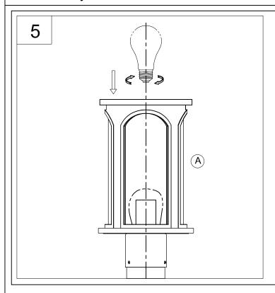
5. Screw lamp (not included) into fixture socket. Use 75-watt MAX incandescent medium base lamp, SBCFL or SBLED.
