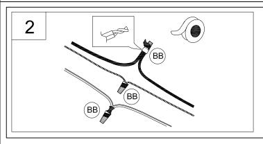
2. Strip  $\frac{3}{8}$ " of insulation from the electrical wire ends. Using wire nuts (BB), connect white fixture wire to the white supply wire from the junction box; connect the black fixture wire to the black supply wire from the junction box.
