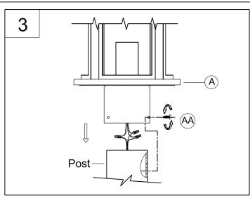
3. Place fixture (A) onto post and use mounting screws (AA) to secure fixture tightly to post using holes drilled in step 1.
