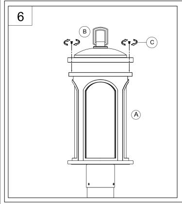
6. Attach the roof (B) onto the fixture (A) and use two flat head screws (C) to secure tightly.
