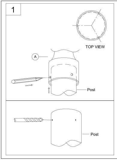
1. Place fixture (A) on post (not included) and use a pencil to mark the locations of the 3 mounting holes. Remove the fixture from the post and use a drill with a 0.144 (4mm) bit to create mounting holes in the post.
